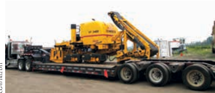
The GT-3400 trimmer is easy to transport. The rear discharge conveyor is positioned to the center of the machine, hydraulically folded, and the entire machine, including trimmerhead, can be driven onto the truck's trailer.
