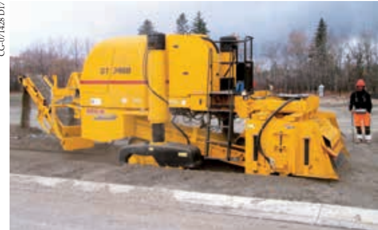
The GT-3400 sidewalk trimmer is operated with a wireless remote control, and its compact size allows it to easily fit between obstacles in zero-clearance sidewalk paving conditions.
