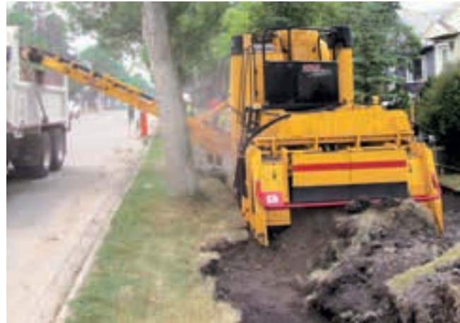
The trimmerhead has a front gate with hydraulic control. The front gate can be raised to trim through windrowed material or lowered for standard trimming applications.
