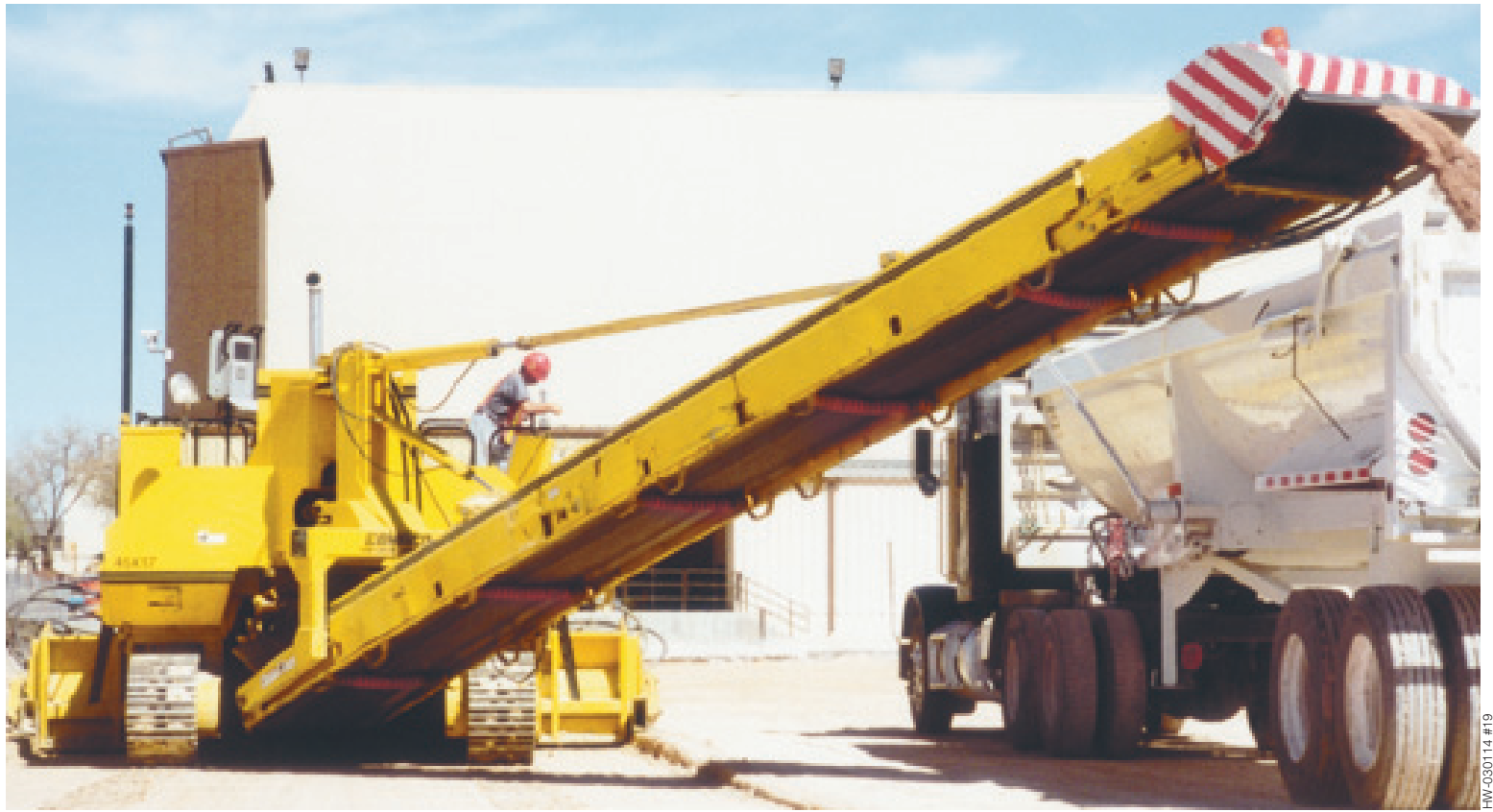
A.S. Horner's 9500 trims the base to grade with the stringless control system.
