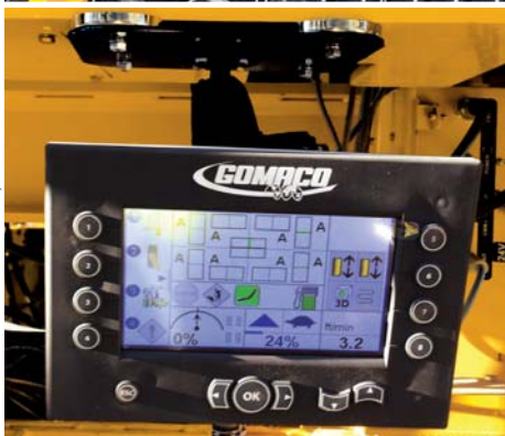
The GP4 was equipped with G+ Ground Control, a remote operator's screen. Ground Control lets the ground crew see the same screen that the operator does at the operator's station. It also allows them to fine tune and make adjustments to the GP4's settings. It can be mounted anywhere on the paver for easy viewing access.
