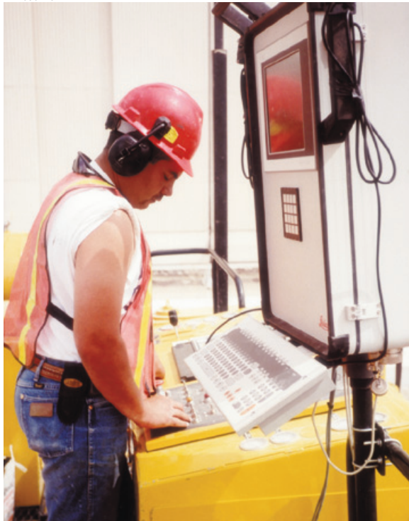
The Command Center is mounted to the GP-2600 next to the GOMACO controller.
