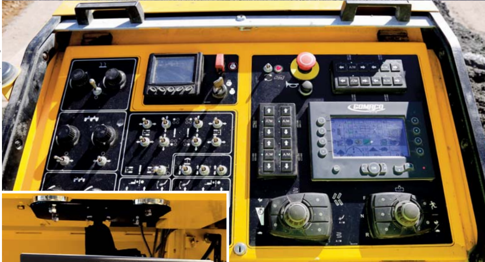
The GP4 was equipped with G+ Ground Control, a remote operator's screen. Ground Control lets the ground crew see the same screen that the operator does at the operator's station. It also allows them to fine tune and make adjustments to the GP4's settings. It can be mounted anywhere on the paver for easy viewing access.
