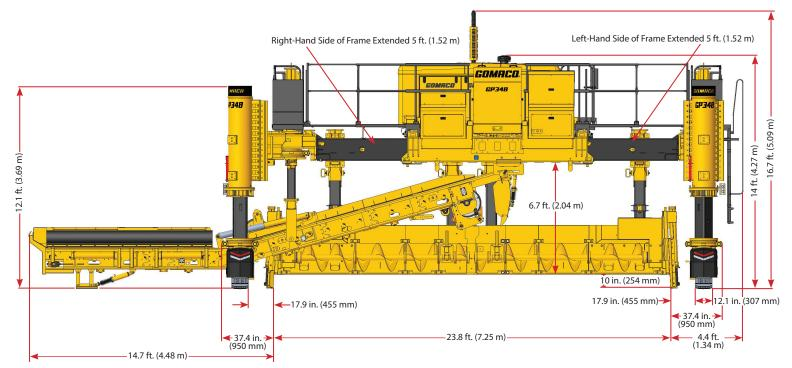
Dimensions are shown at a 24 foot (7.32 m) placing width for two-lane roadway paving. Standard conveyor length is 22 feet (6.7 m).
