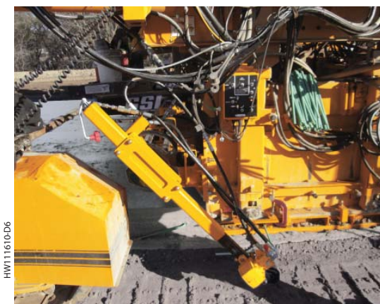
The four-track paver's hydraulic powered bar inserter is located in front of the rear paver leg at the end of the mold.
