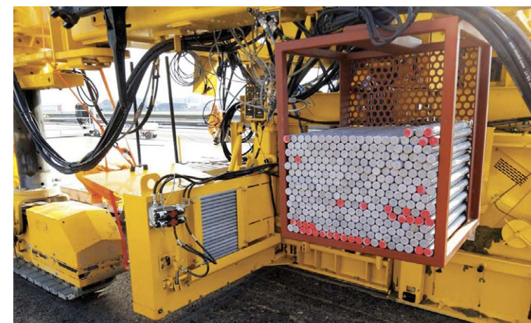
The hydraulic powered magazine-style side bar inserter allows personnel to load multiple bars into a magazine clip, the bar inserter then releases a single bar and places it at the specified distance.
