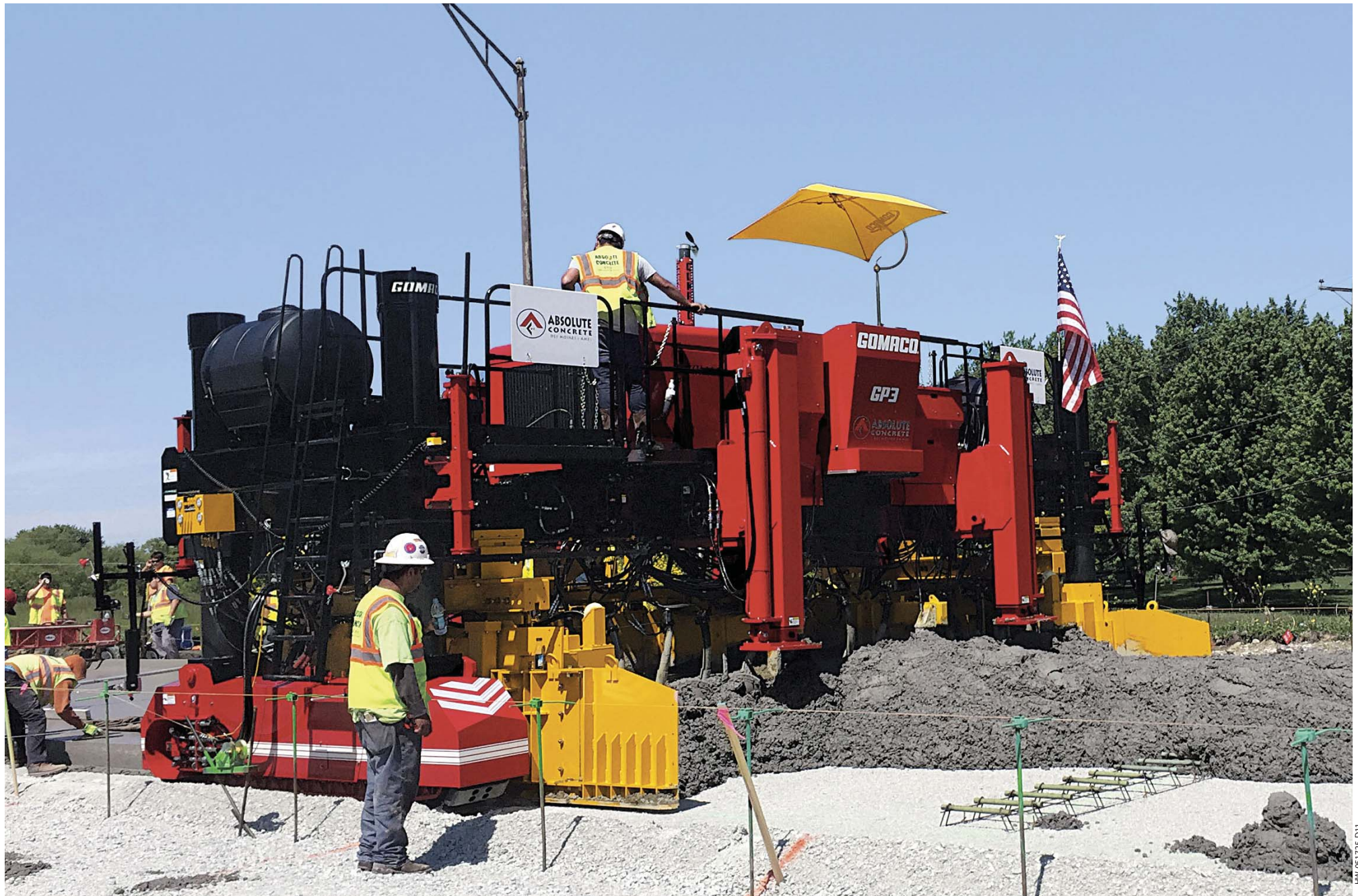
Outriggers can be added to the two-track GP3 for transport loading and frame widening. With the addition of the outriggers, the GP3 can be raised and a truck trailer can be backed underneath the machine.
