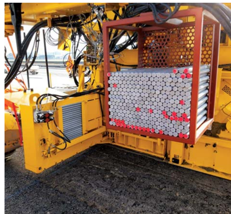
The hydraulic side bar inserter, complete with magazine bar feed, allows personnel to load multiple bars into a magazine clip. The side bar inserter releases a single bar and places it at the specified distance.
