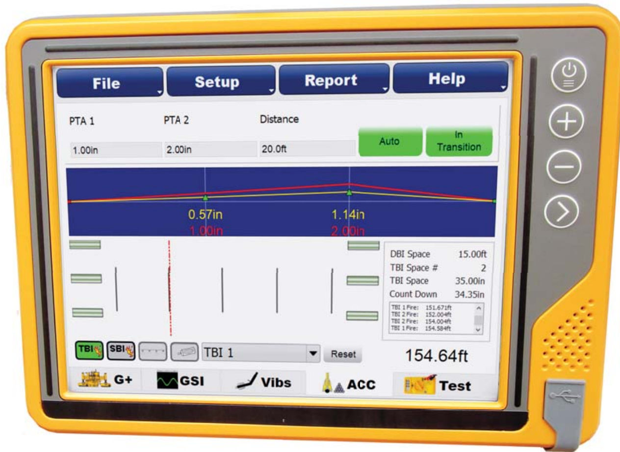
ACC (Accessories) Screen shows how many PTAs, TBIs, and SBIs are set up on the paver, and the distance between them.
