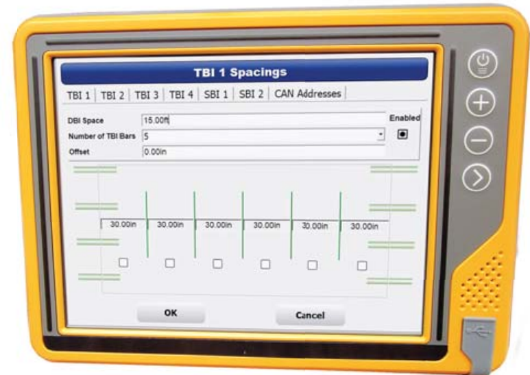
ACC (Accessories) Screen shows how many PTAs, TBIs, and SBIs are set up on the paver, and the distance between them.
