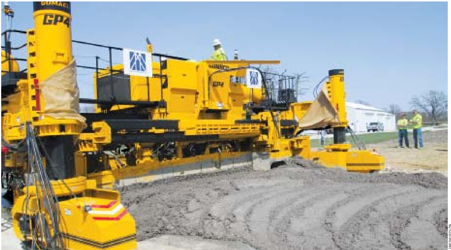
This four-track GOMACO GP4 features a plow on the front to evenly spread the concrete across the paving surface. The GP4 is also equipped with GRD (GOMACO Remote Diagnostics) telematics and diagnostics specifically designed for GOMACO equipment.
