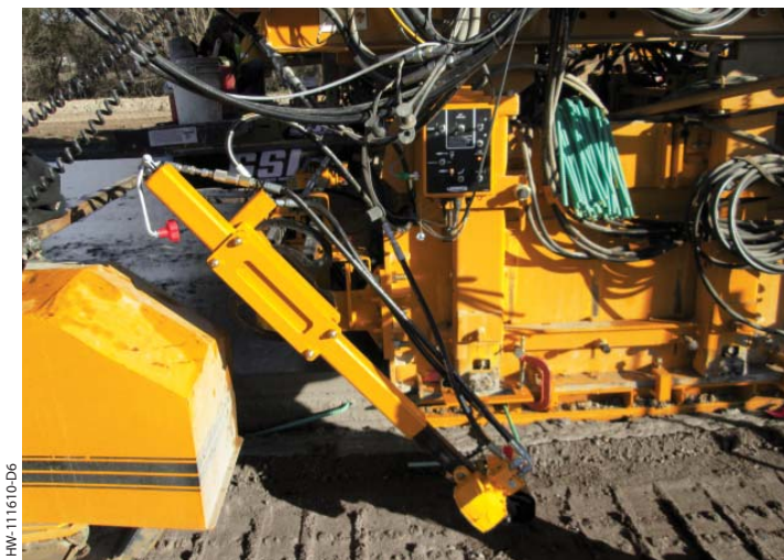
The four-track paver's hydraulic powered bar inserter is located in front of the rear paver leg at the end of the mold.
