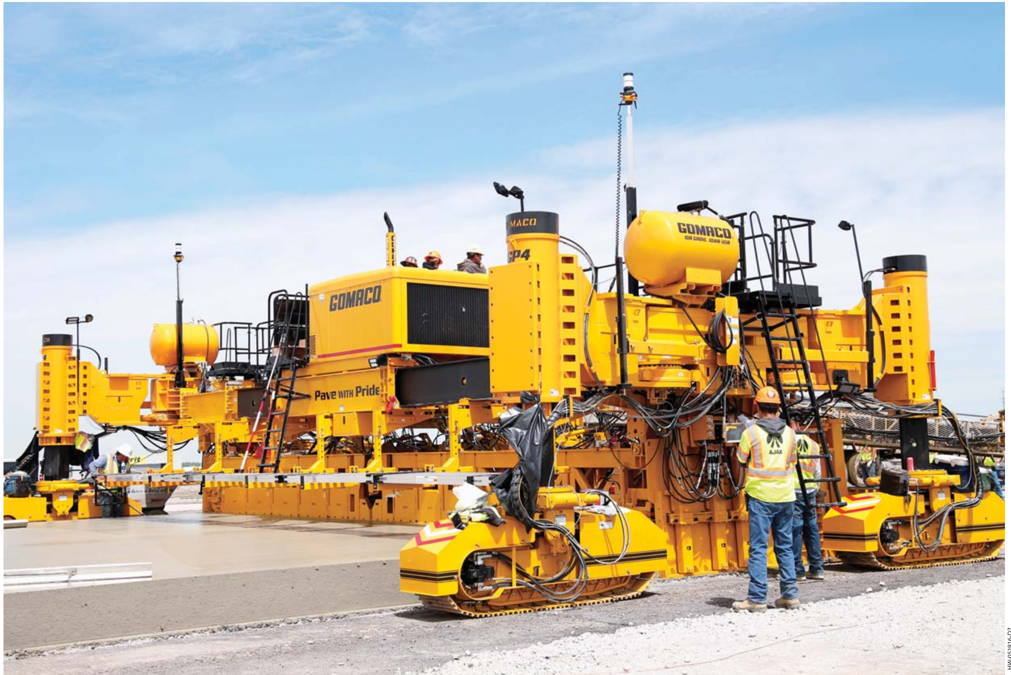
This four-track GP4 is slipforming an airport runway 37.5 feet (11.43 m) wide and 17 inches (432 mm) thick using 3D machine guidance. The GP4 features an aluminum work bridge and is equipped with the 5400 series mold which produces a smooth, clean, and sharp GOMACO edge.
