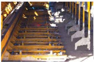
**4:** The patented insertion forks have been designed to provide the industry standard in bar placement accuracy. The holders on the heel and toe of the insertion forks ensure the most accurate bar placement. The fork design and vibration reduces the amount of scarring on insertion and enhances consolidation of material around the bars.
