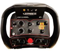
The Radio Remote Control on the CC-1200e provides the operator with full control of the machine while moving around the job site.
