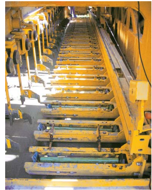
The GHP-2800 was equipped with an IDBI to place the dowel bars for the transverse joints into the new pavement.
