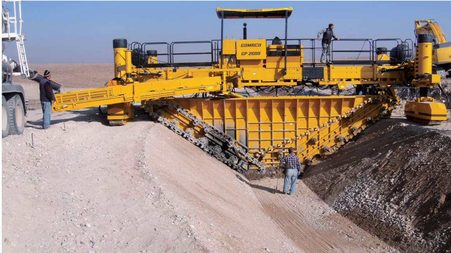
Ready-mix trucks discharge onto the GP-2600's conveyor which dumps into and fills the hopper on the trapezoidal mold. The GP-2600 features a dual-drive chain trimmer with 27 meters (89 ft) of chain and modified teeth to help move the material up the slope of the canal.
