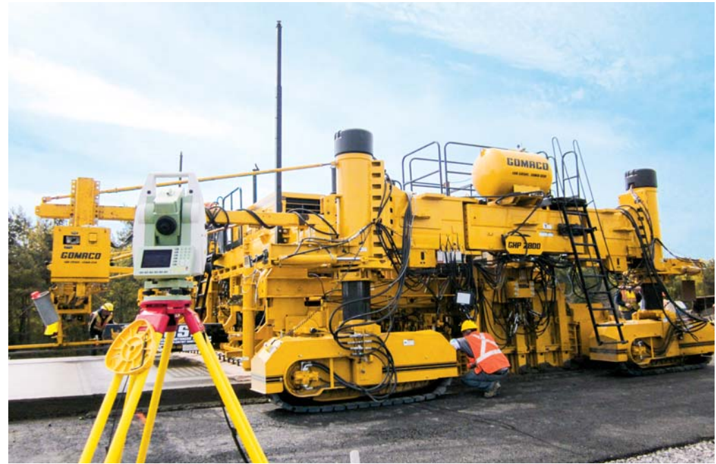
Surianello Concrete is using a Leica 3D stringless guidance system on the GOMACO GHP-2800 four-track paver.
