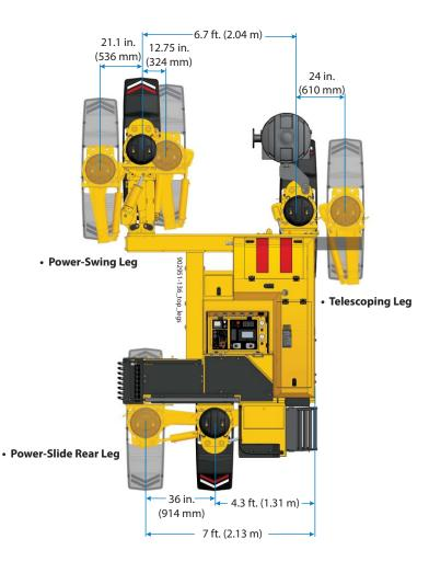
**All-Track Positioning (ATP)** provides the versatility in our slipform pavers. GOMACO's left-front track features a pivoting power-swing, the right-front track hydraulically extends/retracts, and the rear track hydraulically sideshifts. Each leg has a reinforced steel attachment plate that allows extra leg height adjustment. ATP provides the capability of performing various applications and working with differences in grade elevations and unique job-site logistics.
