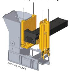
GOMACO's Hook-and-Go mold mount system has no pins or latches and makes it quick and easy to change molds. Simply drive the GT-3600 up to the mold and hook the mount to a special attachment plate. The mold is then hydraulically lifted up and can go to work slipforming the project... just hook and go. GT-3600 molds are built for this system and existing molds can easily be retrofitted in the field.
