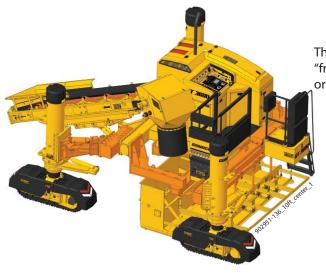
The centermounted mold on the GT-3600 is built with a "frame around a frame" concept, which is illustrated by the orange sections of framework in these drawings.
