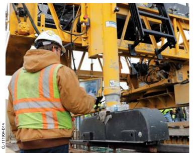
The C-450 and high-production screed can be controlled by a touchscreen on ground level. With the operator being at ground level, they can view exactly what the machine and high-production screed is producing so they can control how far to advance it or what changes need made during the paving process.
