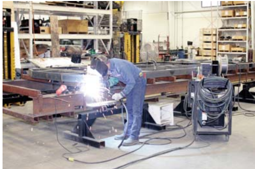
Certified welders build the trolley's frame.
