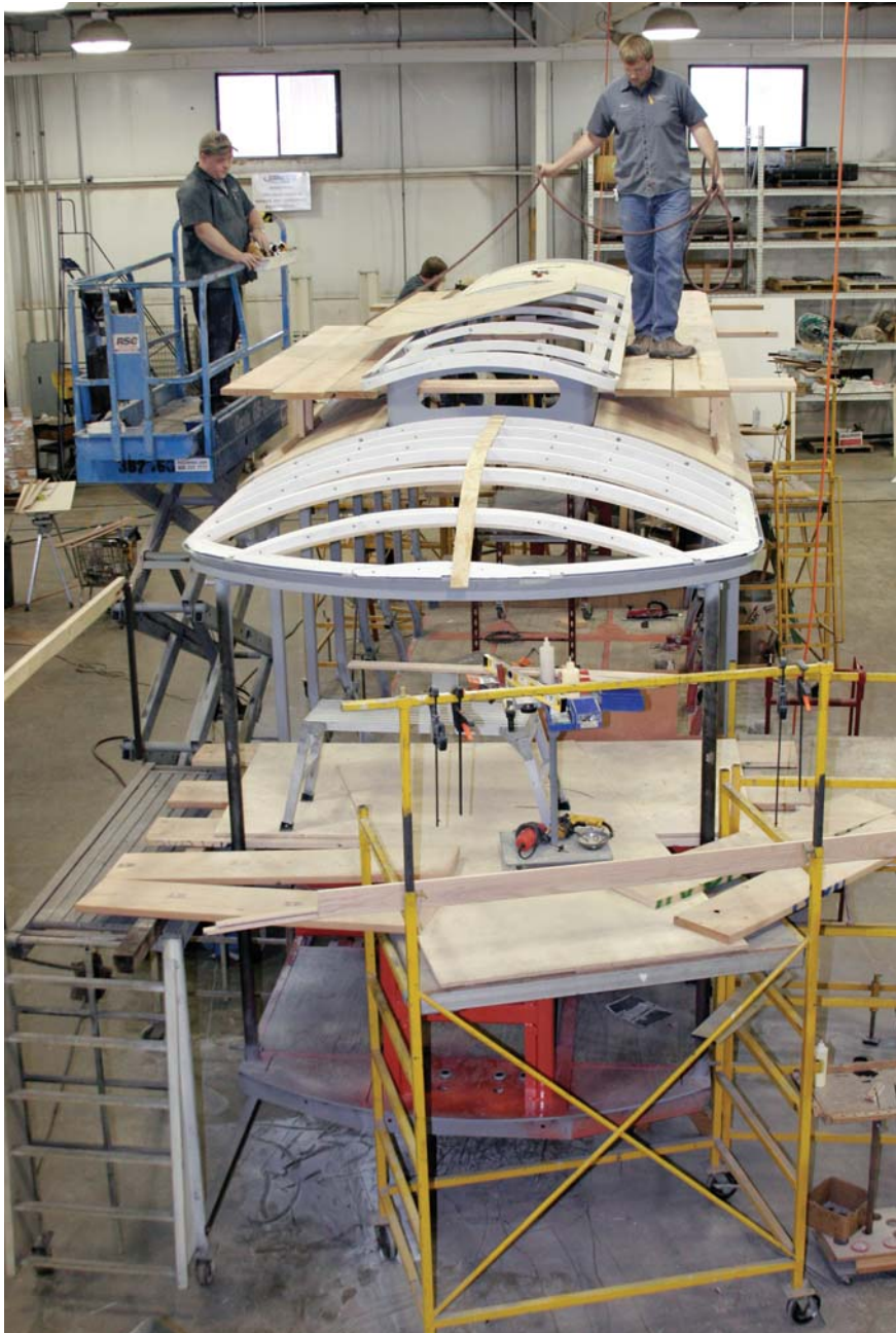
Scaffolding surrounds the steel shell of what will be become Trolley #1717.
