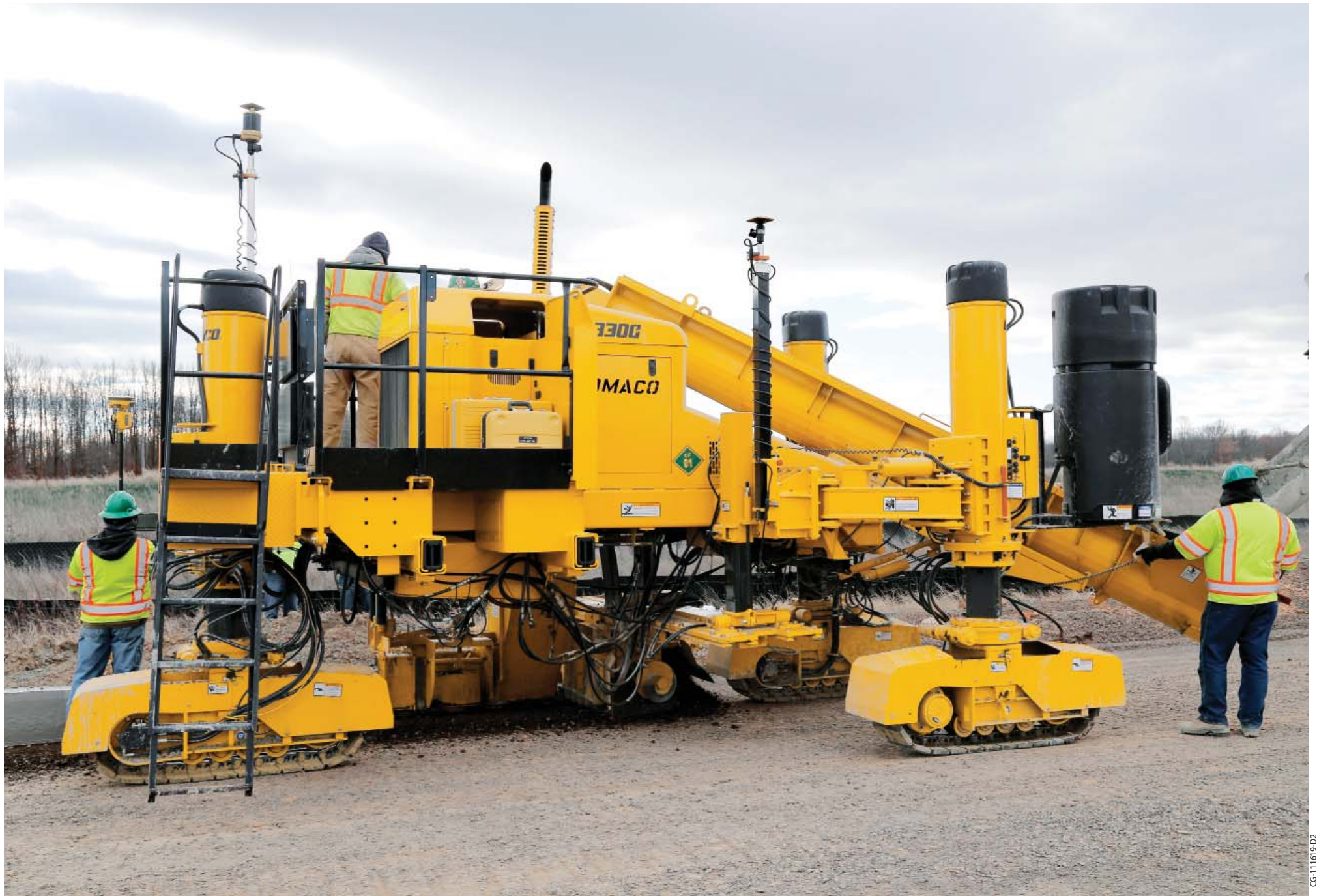
The GOMACO 3300 is designed for right-side and left-side pours. The U-shaped operator's platform and sliding console allow for optimum visibility and control to pave in either direction.
