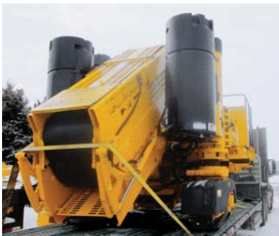
The folding conveyor reduces the transport dimensions on the GOMACO 3300.
