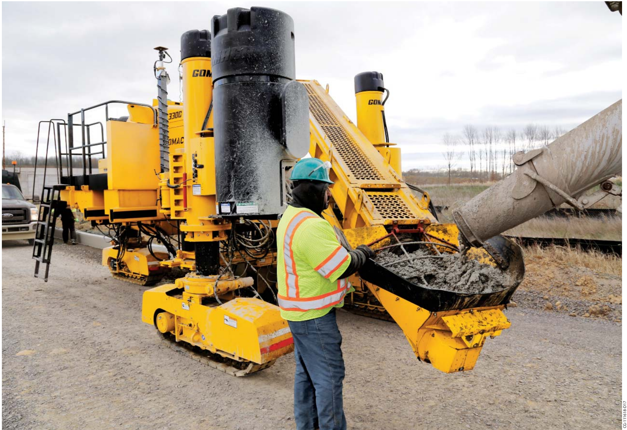
The charging auger on the 3300 is equipped with vibration to release concrete build up from the safety guard at the end of the hopper. The auger's safety guards are hinged to allow for cleaning.
