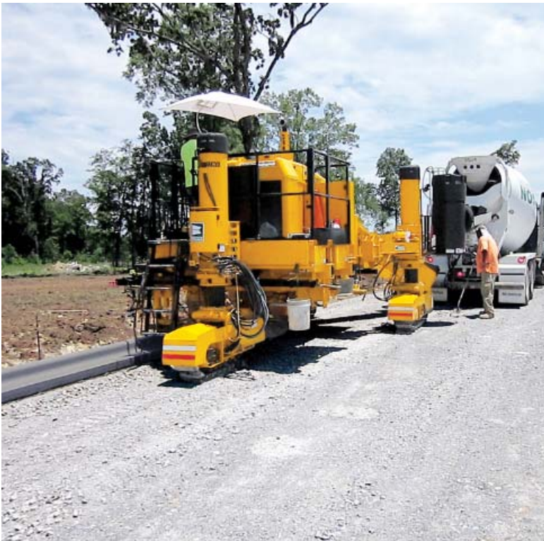
The GOMACO 3300 features the power-slide rear leg to position the leg for weight distribution.
