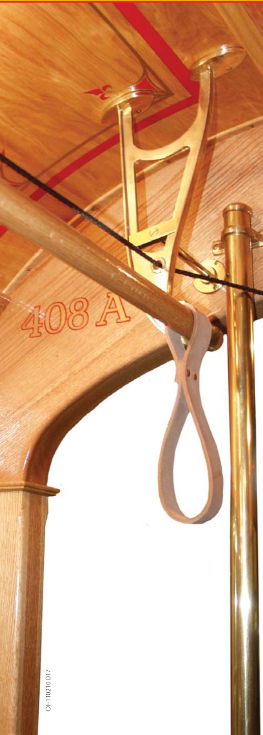
Brass fittings across the top of these benches allow passengers to switch the bi-directional benches according to the direction of trolley travel.
