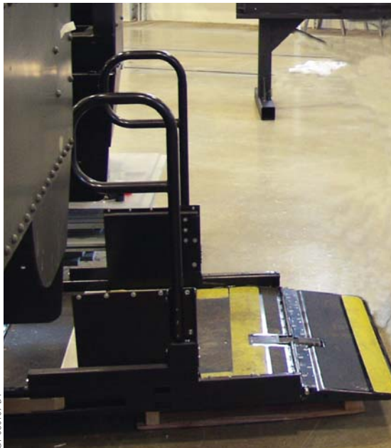
The wheelchair access ramp folds down during testing to allow handicapped accessibility.
