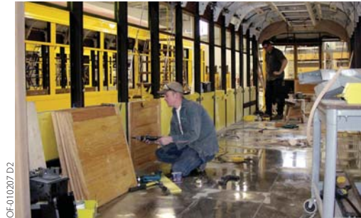
The Birneys feature a ply-metal flooring, which is a layer of 0.75 inch plywood sandwiched between layers of stainless steel. The ply-metal is both water and fire resistant.
