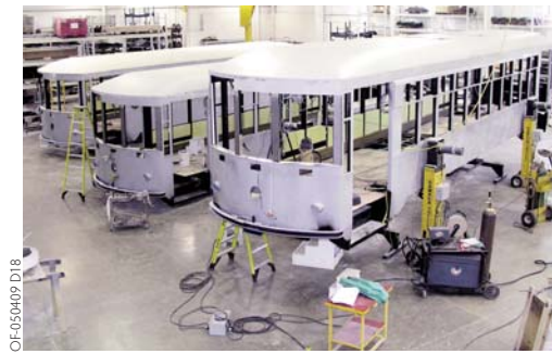
Certified welders build the trolley's frame.
