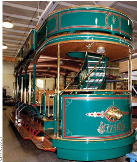
Los Angeles, California - Refurbishing project which included total repainting, refinishing the original woodwork, new flooring and steps, new brass handrails, rewiring the controls, and installing the Gomaco proprietary K35G controller.
