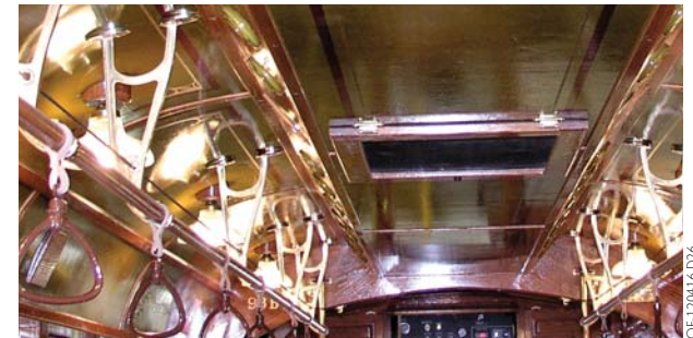
Glossy brass fixtures created in the Gomaco Trolley foundry support the handrails and grab bars helping ensure rider safety.
