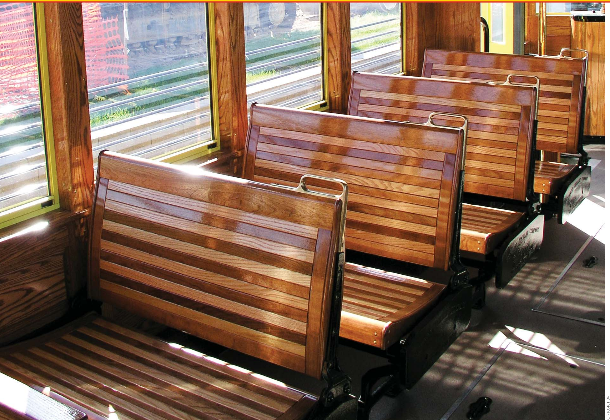
Only the finest, premium lumber is used in a Gomaco trolley. These benches are made from alternating oak and cherry hardwoods, built and finished by Gomaco's talented craftspeople.
