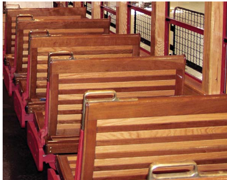
Brass fittings across the top of these benches allow passengers to switch the bi-directional benches according to the direction of trolley travel.
