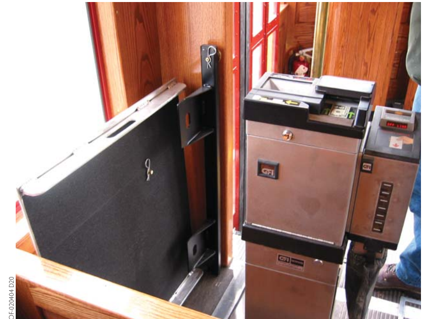
An interior view of the wheelchair ramp and control system is shown on the replica Birney trolley in Memphis.
