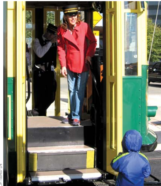
The wheelchair ramp forms into steps for the general public when retracted.
