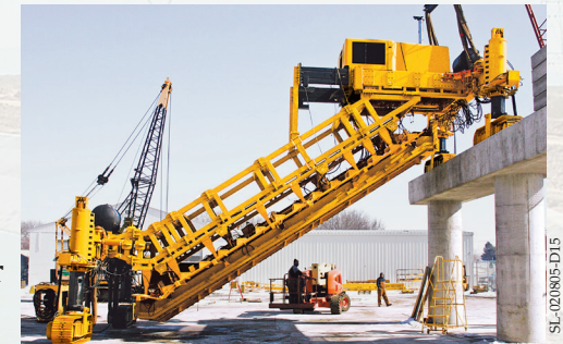
GOMACO built a concrete testing pier at their facilities to test the canal equipment.
