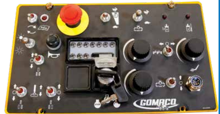
Travel, grade, vibrators, and auger controls are located on the handle for easy reach.
